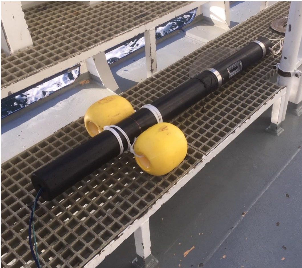
Figure 19 - Stereo Catch Monitoring Probe (S-CMP) ready for deployment during the research cruise on M/F Fiskebas. The floatation section and the camera section are connected, with the support line and cable pass through the float so that the depth of the camera relative to the surface can be controlled. This version is fitted with an Ethernet cable, for direct camera feed from the probe, as well as additional weight and floatation to stabilise the camera's vertical position in the water.
