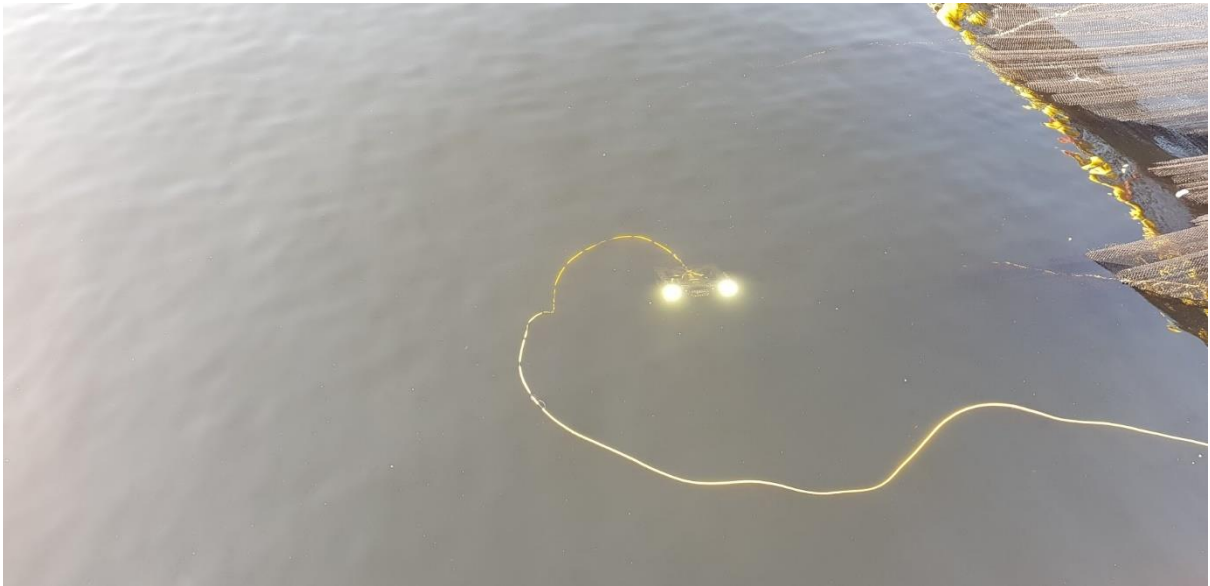
Figure 18 - ROV ("FishBot") inside purse seine with lights on.
